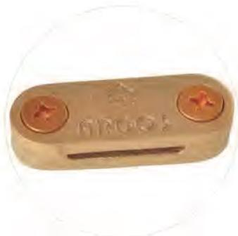
Metallic DC clips secure the flat tape conductor to the building surface. Fix using countersunk woodscrew 1 1/2" x No. 10 and No. 10 wall plug.
